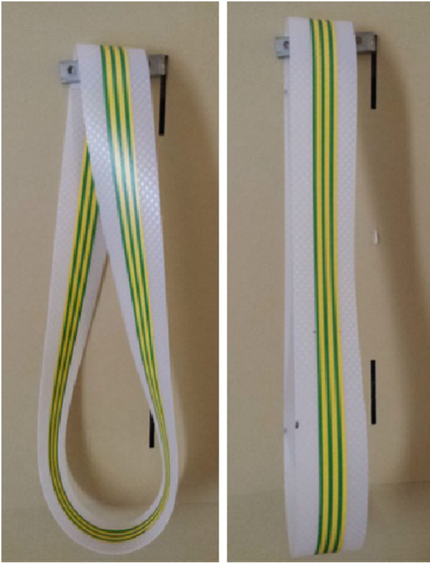
Figure 8. Juxtaposition of how a belt with normal two-sided topology hangs from a pulley to how a Möbius strip hangs; compare with Figures 6 and 7.
